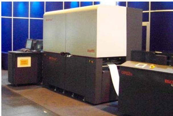
Modularity and flexibility are inherent in the new generation paper transport bases, designed to meet the most demanding applications for Mono and Colour digital printing systems. As a modular system the unit can be configured for 1, 2, 3 and 4-up documents, for simplex or duplex printing applications.
