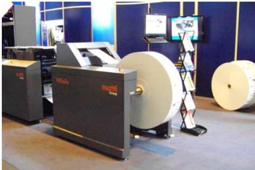
By utilising the options package the rewinder can be configured for a vast range of printer. All the rewinders incorporate a soft start system, therefore ensuring reels are consistently rewound to pre set tension parameters. Thus ensuring the reel is wound to the highest standards, which is crucial for subsequent processing.
