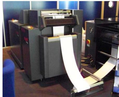
The New Buffer Accumulator is a multi function device, which allows pre and post processing equipment to be connected to the most demanding printer and is capable of storing up to 6 metres of paper in a small footprint.
