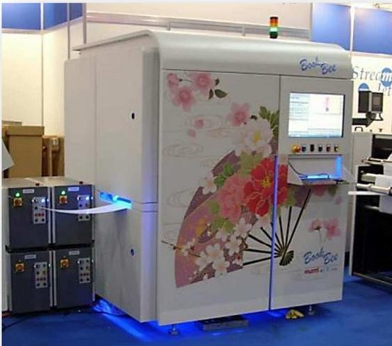
The digital printer has been developed to print duplex without the need for turner bars. The **CTC Digital Press** was printing 600 x 600 dpi using Piezo Drop on Demand technology. The printer incorporates built-in UV drying featuring LED pinning and standard UV final cure.
