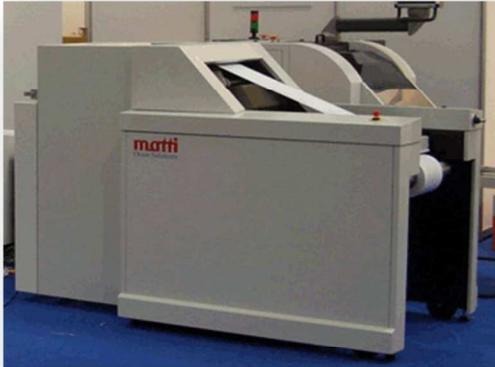
By utilising the options package the rewinder can be configured for a vast range of printers or other host devices. All the rewinders incorporate a soft start system; therefore ensuring reels are consistently rewound to pre-set tension parameters. Therefore ensuring the reel is wound to the highest standards, which is crucial for subsequent processing.
