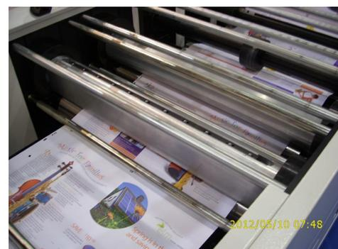
At Drupa the **MFP** was shown producing Sprocket Holes Post Printer, Coupon and Giro application all controlled via the 2D code.
