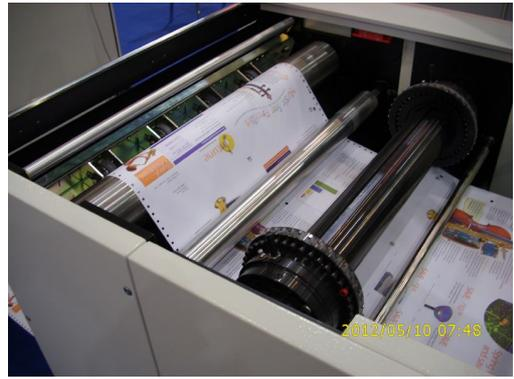
Processed exhibition application showing File Hole Punching Coupon Perforation and Sprocket Punching
