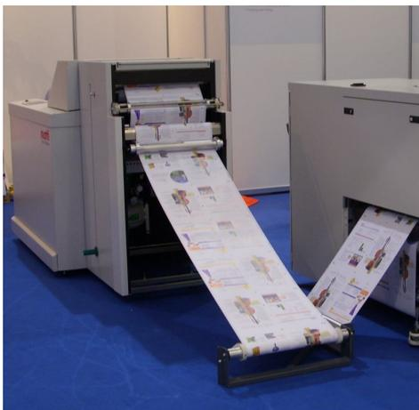
By utilising the options package the rewinder can be configured for a vast range of printers or other host devices. All the rewinders incorporate a soft start system; therefore ensuring reels are consistently rewound to pre set tension parameters. Therefor ensuring the reel is wound to the highest standards, which is crucial for subsequent processing.
